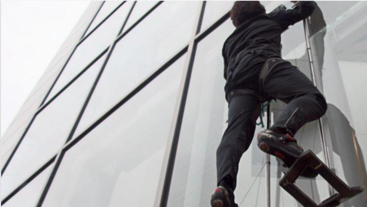
Stanford graduate student Elliot Hawkes demonstrates a new hand-sized gecko-inspired adhesive device that allows a human to climb a glass wall like a gecko. (Elliot Hawkes, Biomimetics and Dexterous Manipulation Lab Center for Design Research, Stanford University)
